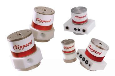
The NIV series media isolation valve is a solenoid-operated device that utilizes a flexible diaphragm to isolate the actuation mechanism from the fluid path. This unique, multifunctional valve stem results in a simplified design with fewer parts, longer life and minimal dead volume. In addition, all wetted areas of the NIV series are PTFE, making it ideal for use with corrosive media.
